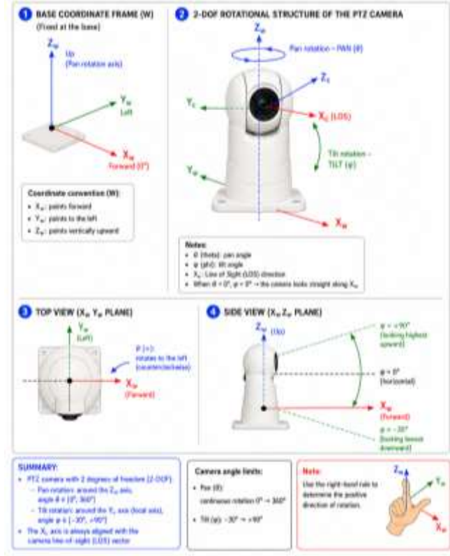
Figure 1. PTZ camera model and frame of reference.
