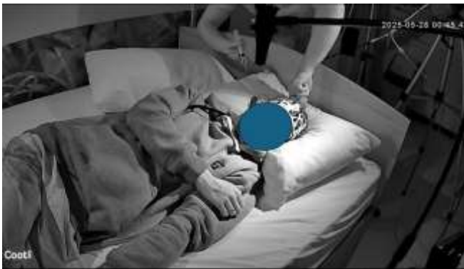
Fig. 2. An example of a frame from a standalone camera. The subject is wearing an EEG cap and two fitness trackers. A microphone is located at the top, used to record the subject's breathing. The subject is asleep, and a nurse is adjusting the amount of conductive gel in the cap
