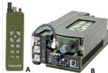
Fig. 20: A) AN/PRC-154A Rifleman Radio: three antennas according to frequency range 225-450 MHz, 1250-1390 MHz, and 1755-1850 MHz; but not just a single smart antenna; B) AN/VRC-121(V)1 VIPER Vehicle Integrated Power Enhanced Rifleman [22]
