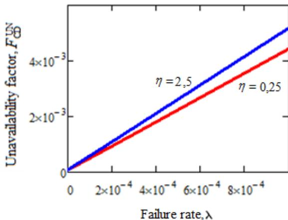
Figure 5. Dependence of the unavailability factor of an optical cable for the degradation cycle on sudden failure rate
