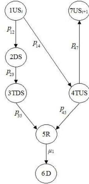
Figure 1. Diagram of state-transitions on one testing period
