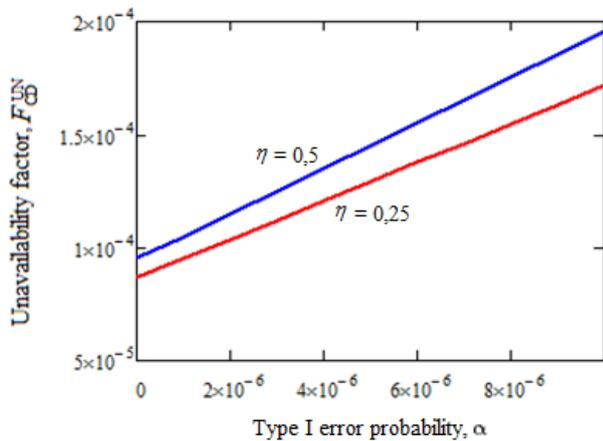
Figure 4. Dependence of the unavailability factor of an optical cable for the degradation cycle on type I error probability
