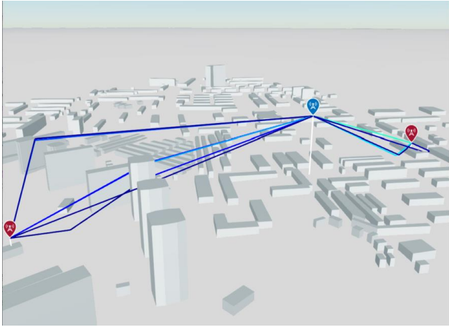
Figure 1. The signal propagation paths between one receiver and two transmitters in a 3D environment
