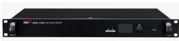
Figure 2. PA System Network Controller
