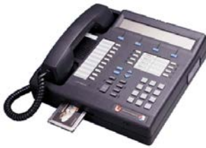
Fig. 9: STE desk set. Note the slot in the front for Crypto PC Card
