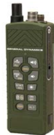
Fig. 3: AN/PRC-154A Rifleman Radio [9]: three antennas for three frequency bands but not a single software-defined antenna as planned [4]
