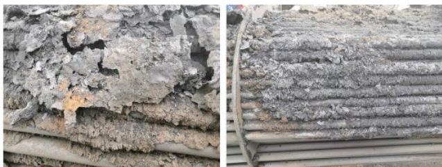
Fig. 2 Deposits on the surface of heat exchanger tubes
