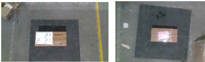
Fig. 8. a. On the left - correct camera angular which leads to correct calculations. b. On the right - displaced camera angle since October 2020 that led to exceeding 2 cm SLA error rate. Source: Authors own elaboration.
